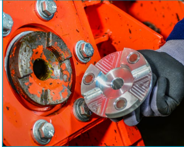
Tool with suitable profile for quick coupler
